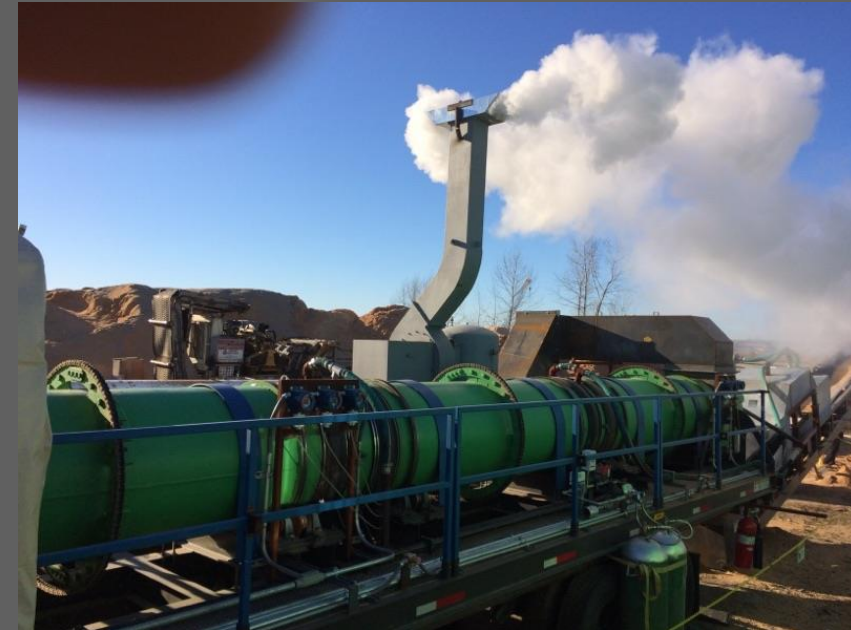
Chemical drying of microchips and pellets. DRYMAXZ System, Biofibre, BC. USFS grant assisted scoping technology for adoption in Idaho.
