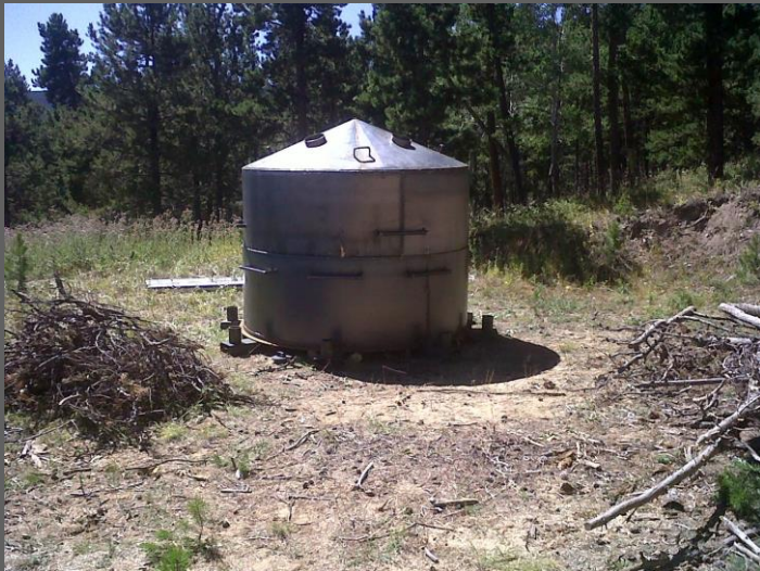
Mobile pyrolysis unit. Amaron Energy, Utah.
